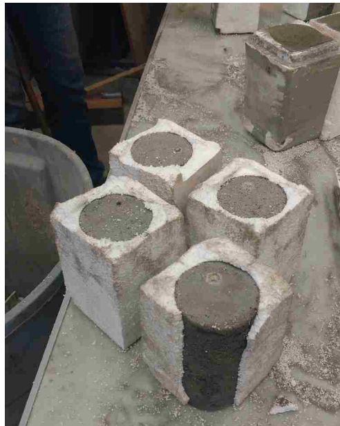
Figure 4-4 : Extraction of cellular concrete cylinders from foam molds.
