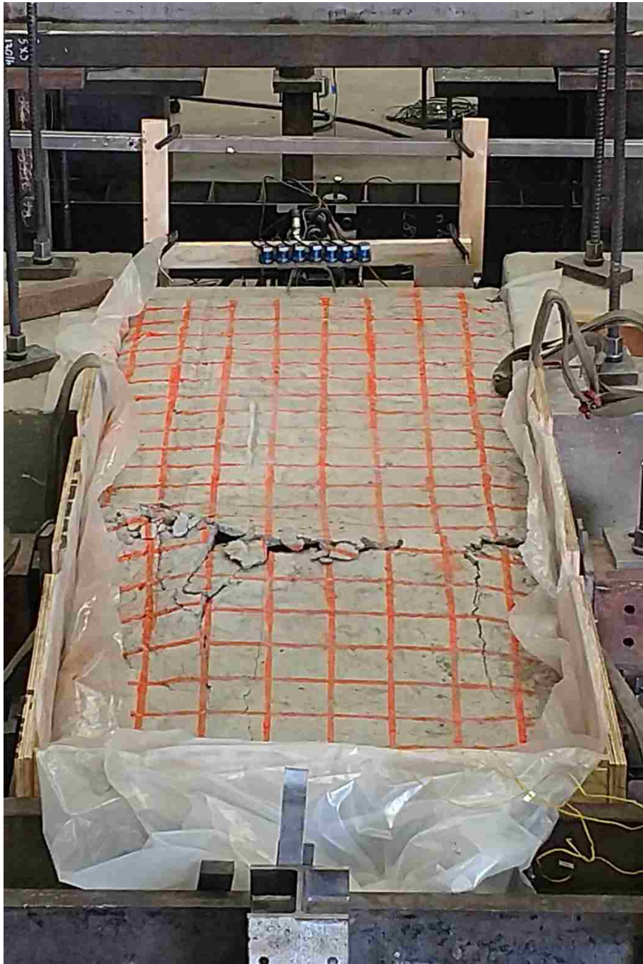
Figure 5-5: Failure surface of the 0° skew test.
