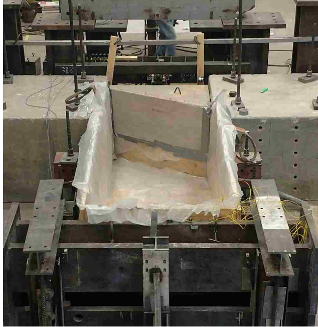
Figure 3-3: Photo of 30° skew test box layout before LCC backfill.
