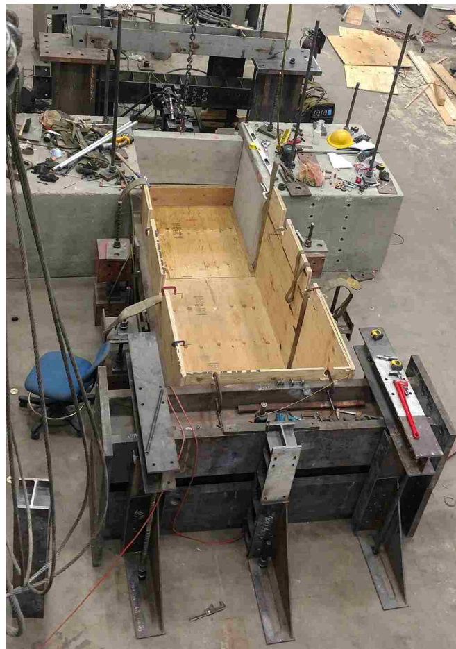
Figure 3-2: Photo of 0° skew test box layout without plastic sheeting.
