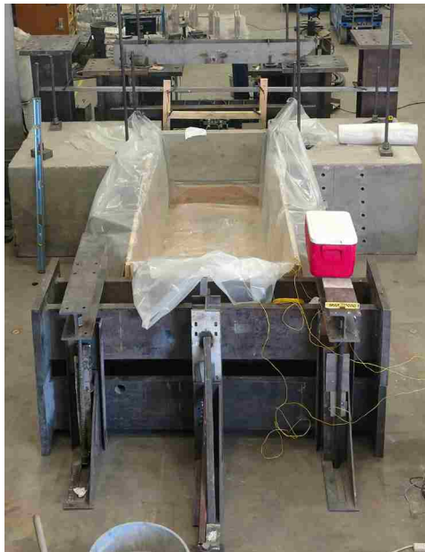
Figure 3-1: Photo of 0^\circ skew test box layout before placement of LCC backfill.
